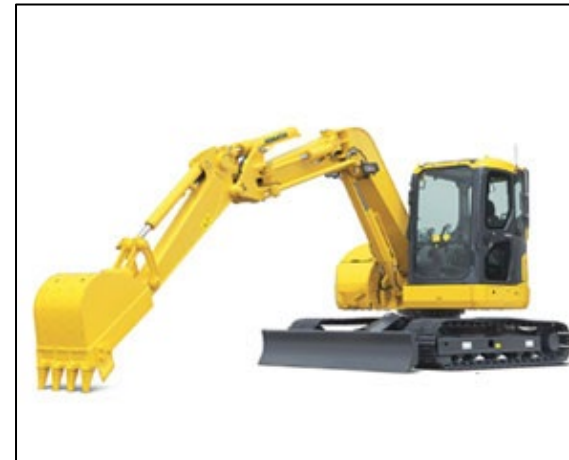
KOMATSU EXCAVATOR, 2.4M WIDE, 8 TONNES
