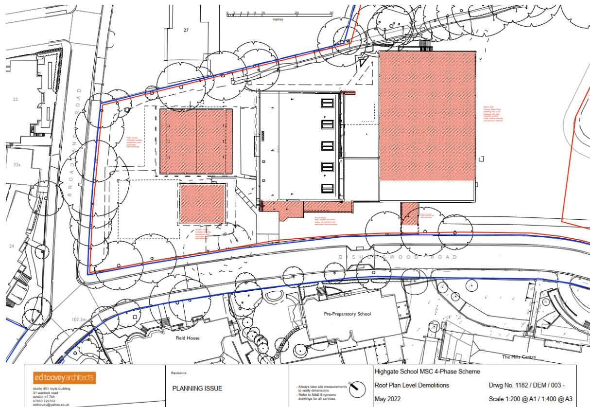
Figure 8 Roof Demolition Plan
