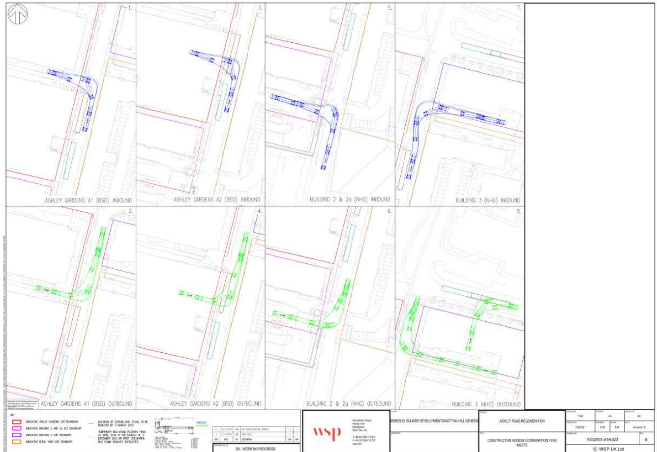
Figure 4-6 – Low Loader accessing the site
