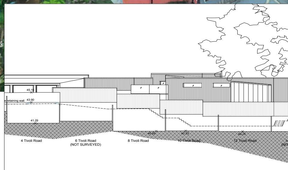
17. STEPPED WALL AND FENCE - TIVOLI ROAD HOUSES
