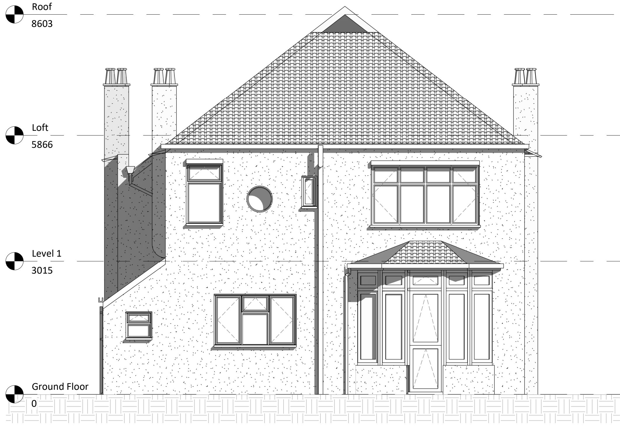
Existing North-East Elevation
