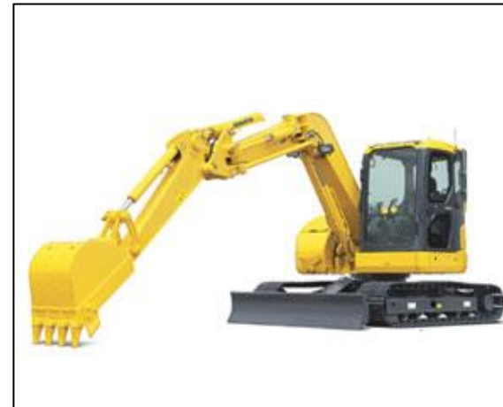
KOMATSU EXCAVATOR, 2.4M WIDE, 8 TONNES
