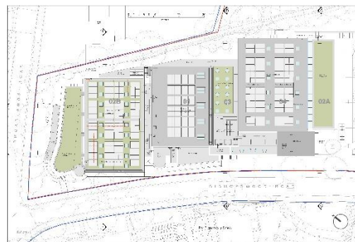
Roof plan proposed showing green roofs with photovoltaic panel arrays
