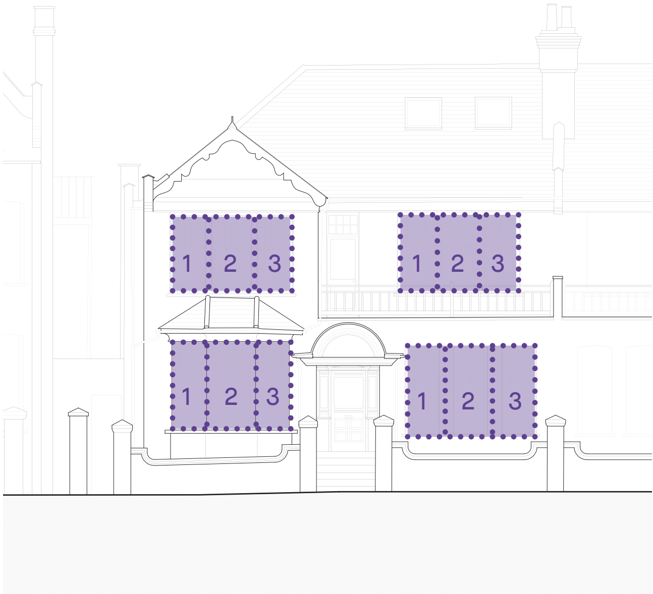
EXISTING NORTH ELEVATION - TRIPTYCH PROPORTIONS
