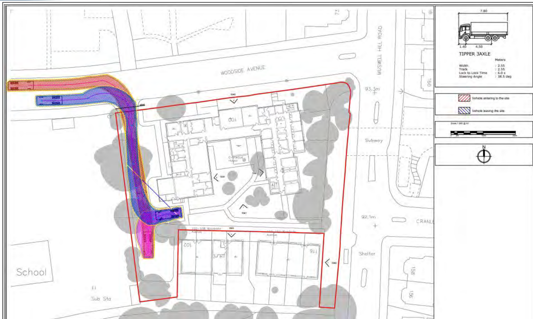
Figure 7.2: Demolition Vehicle Access and Egress (Muck Away)
