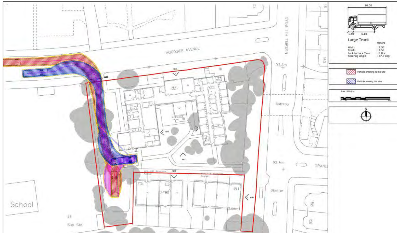
Figure 7.1: Demolition Vehicle Access and Egress (LRIGID)
