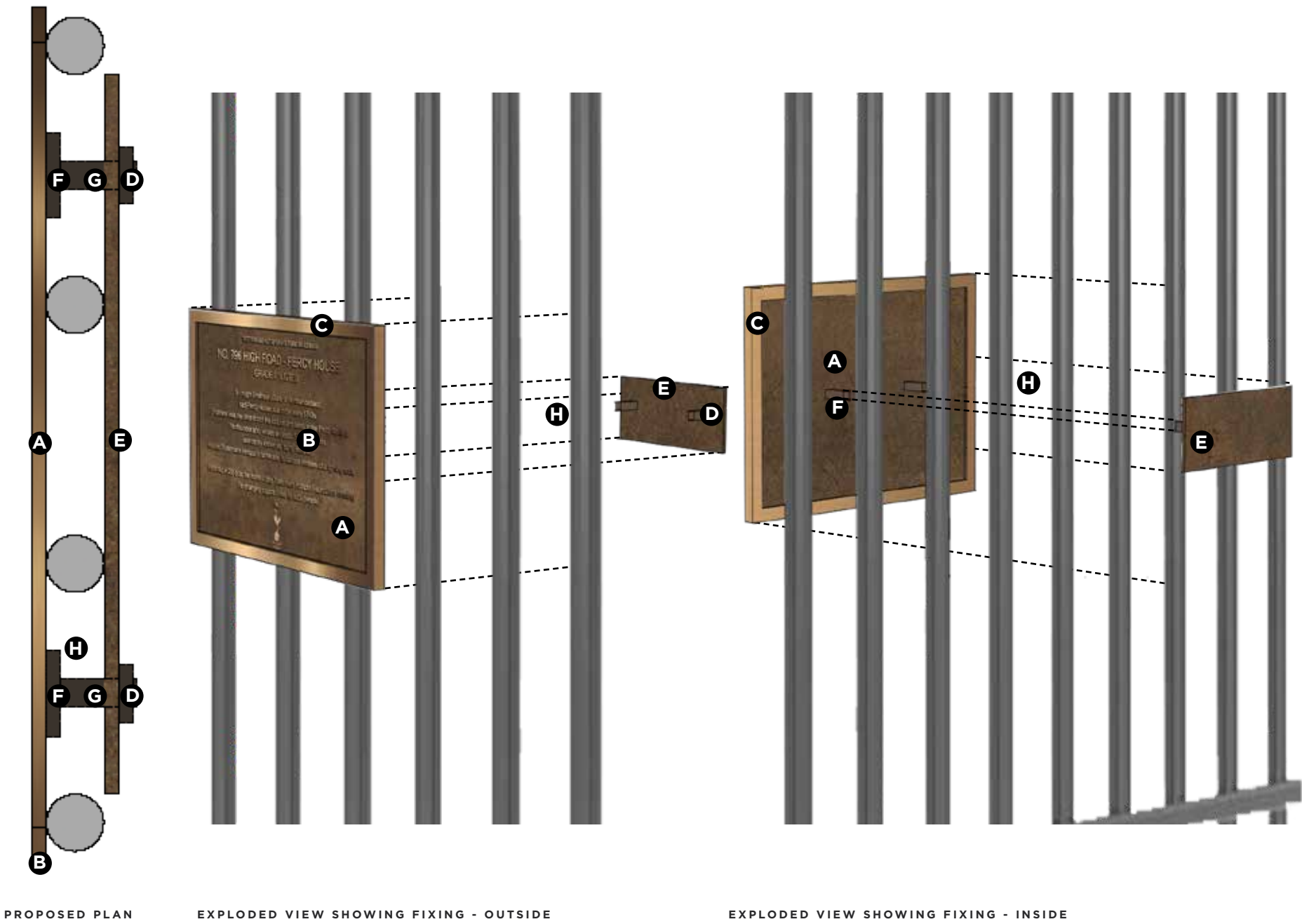
FIGURE 33. - Proposed Fixing Methodology
