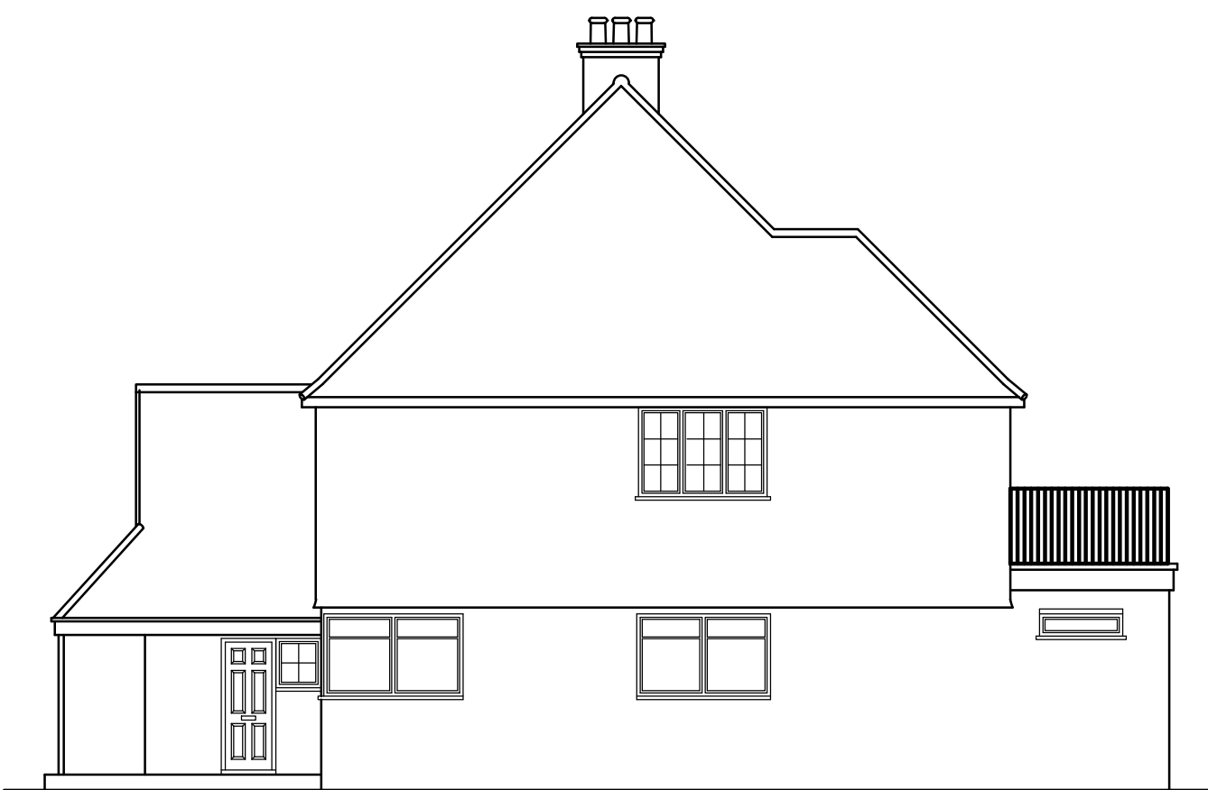
EXISTING SIDE ELEVATION 1:100
