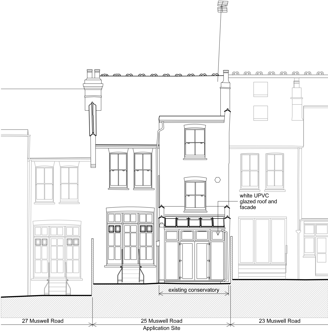
EXISTING REAR ELEVATION
