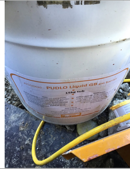
Pudlo Liquid Gas Barrier used on
