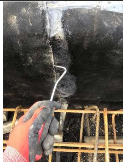
Additional pick and probe test carried
