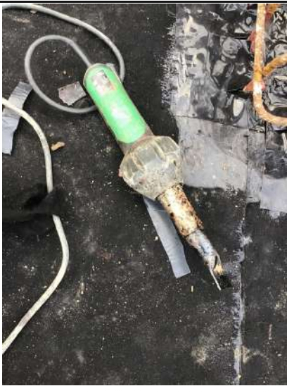
Hot air leister used to weld laps of the
