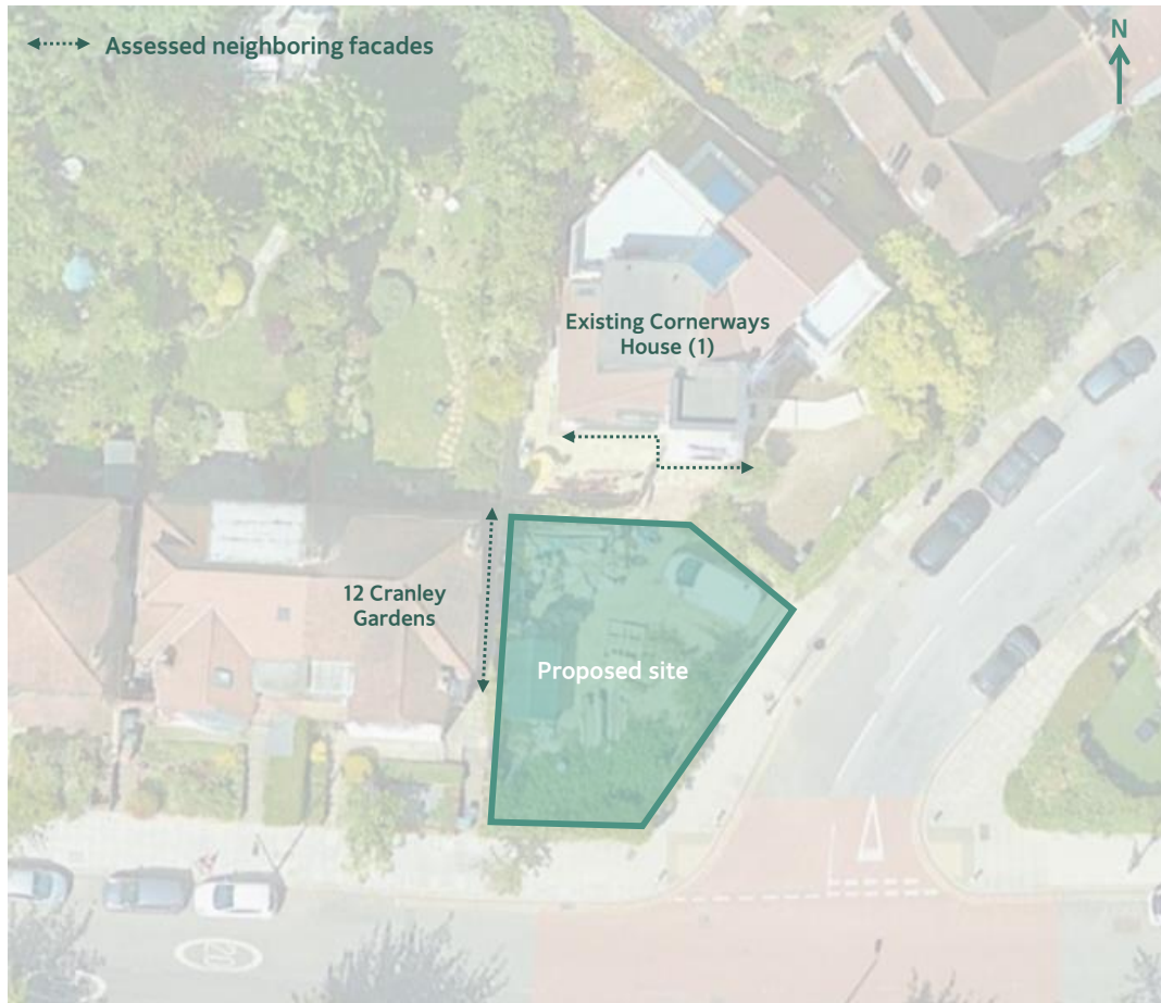
Figure 6: Daylight assessment - neighbouring property façades
