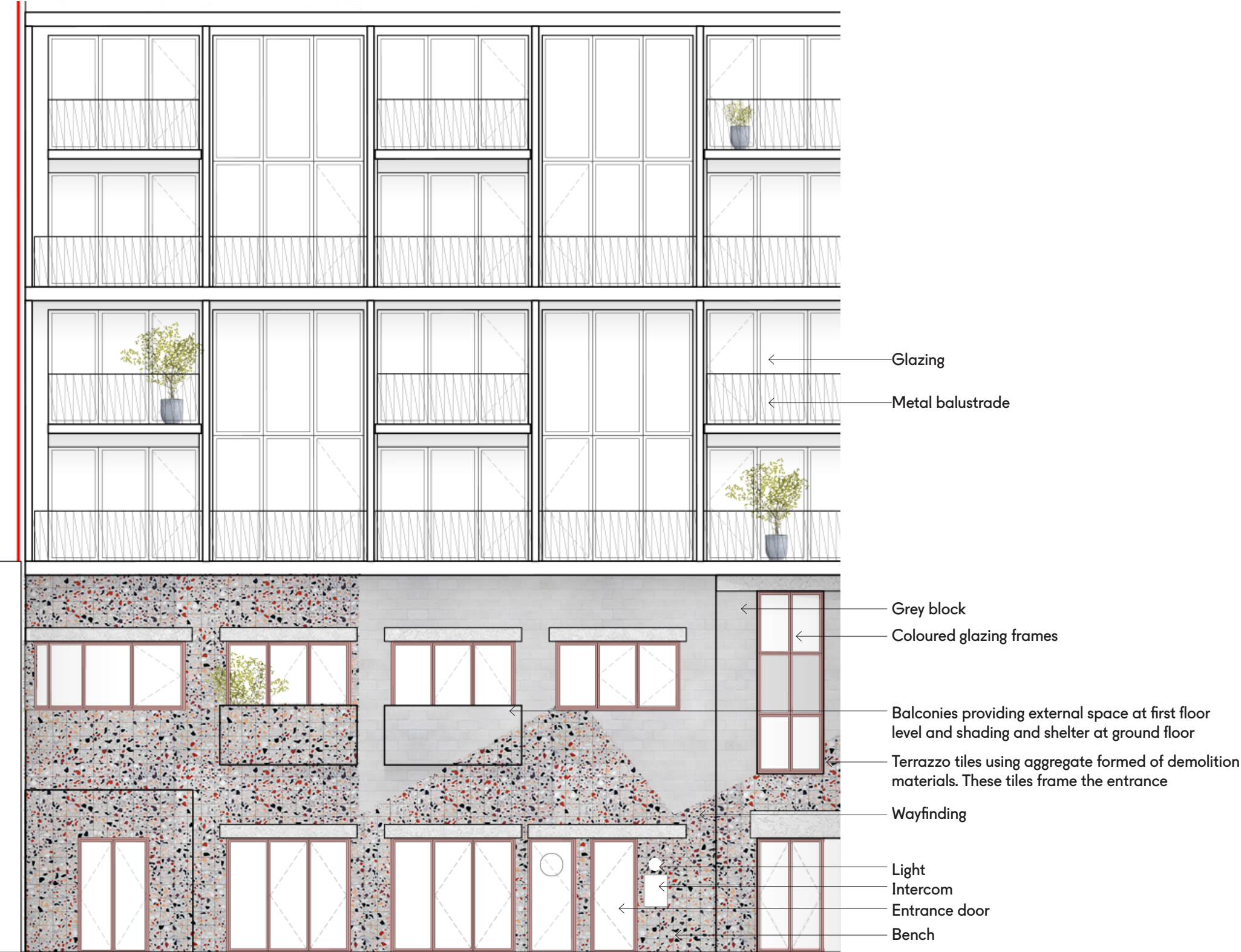
Typical Courtyard Elevation
