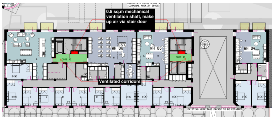
Figure 8: First Floor smoke ventilation strategy
