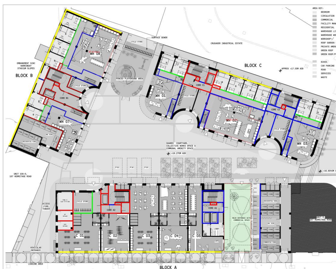
Figure 16: External Fire Spread Analysis
