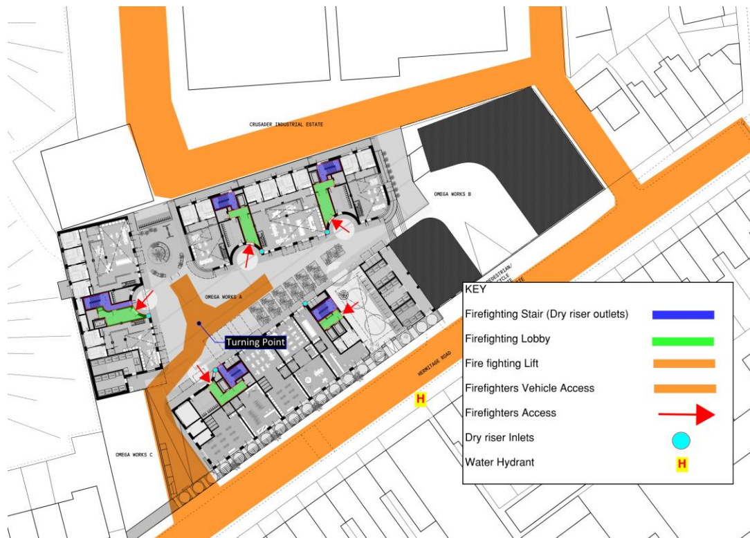
Figure 17: Fire Service Access and Hydrant Location
