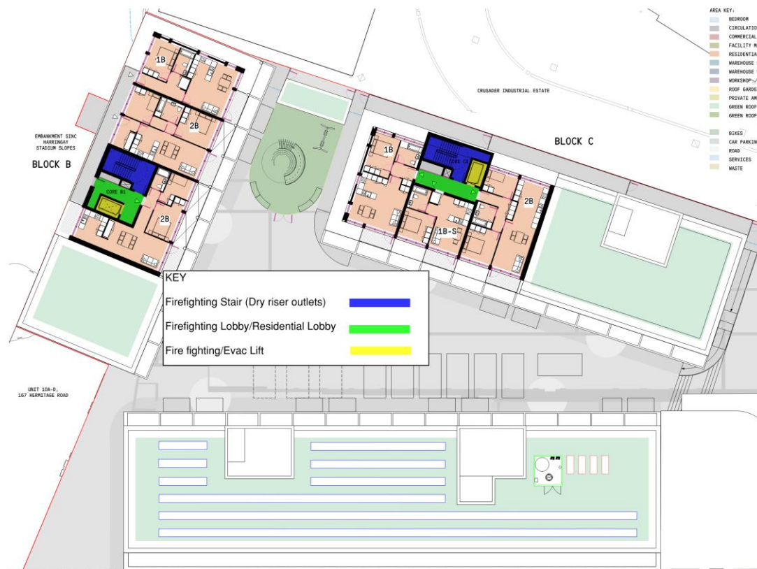
Figure 8: Firefighting shafts and Evacuation lifts
