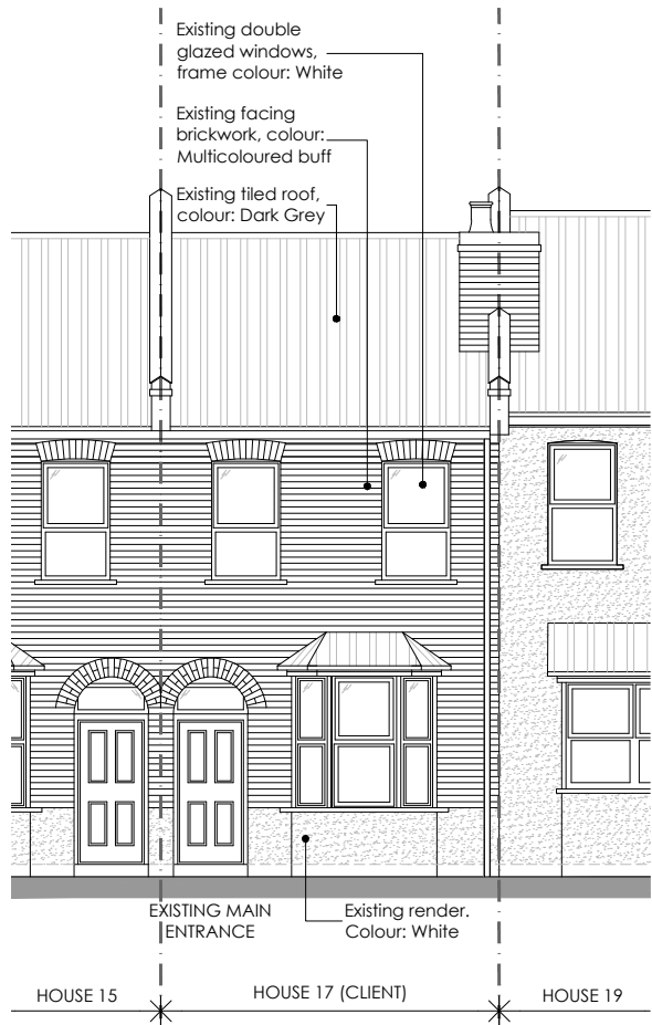
EXISTING FRONT ELEVATION
