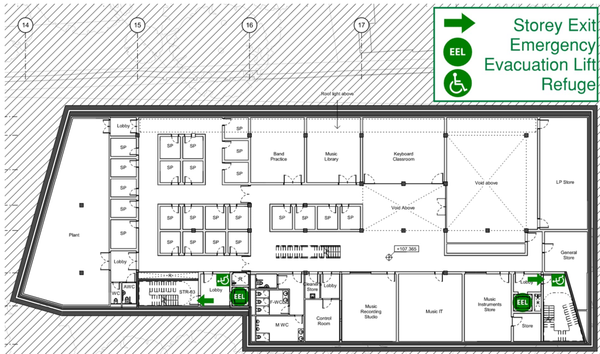
Figure 4: Classrooms Means of Egress from level -05
