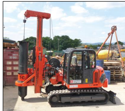
CF3 RIG, 2.2M WIDE, 11 TONNES
