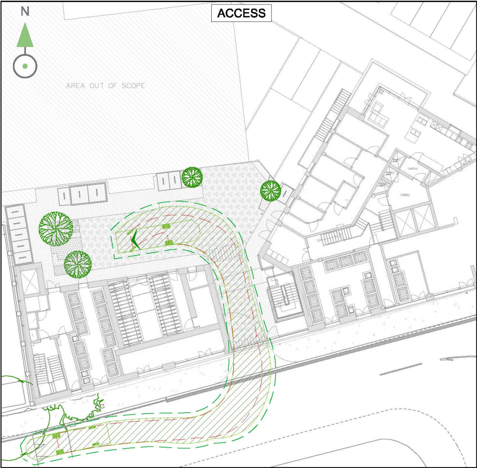
Ground Level - Fire Tender Access
