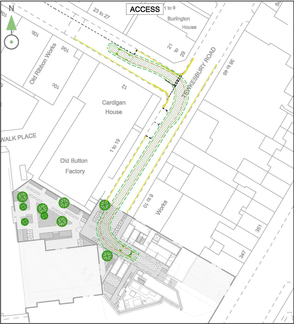
Tewkesbury Road Level - Fire Tender Access
