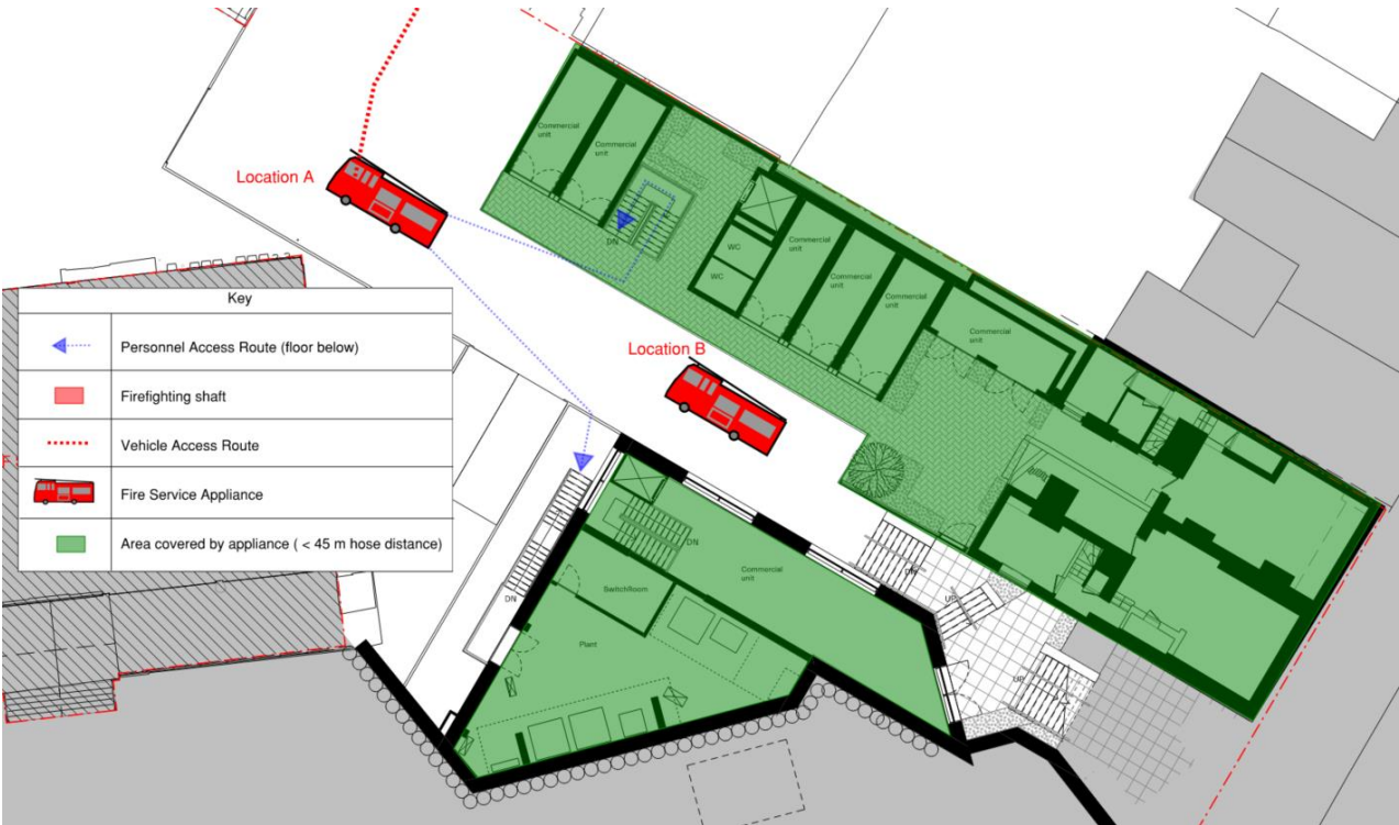
Figure 7.10 Indicative plans that show Tewkesbury mezzanine access
