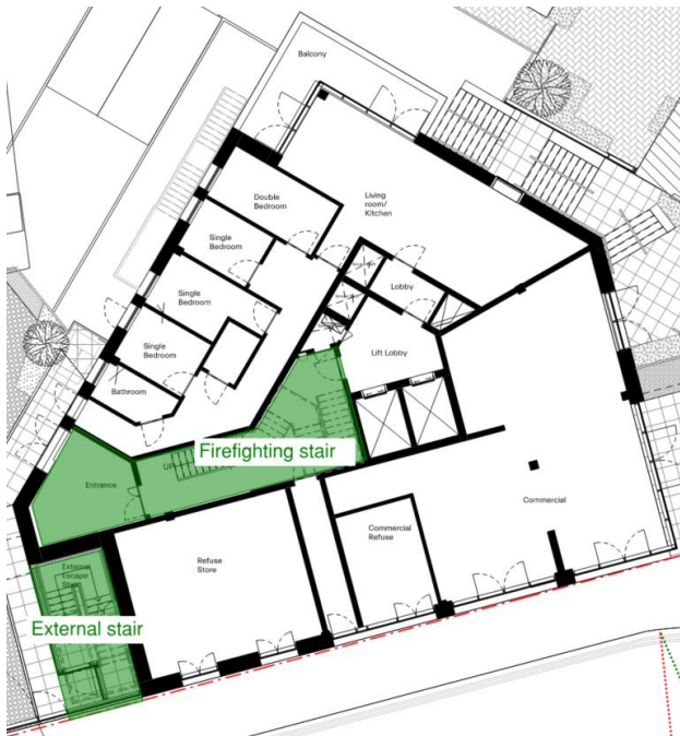
Figure 2.3 Stair location (Block A)
