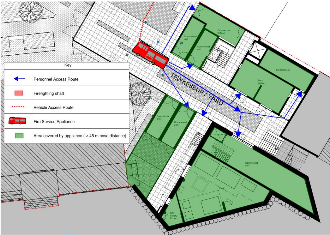
Figure 3.1 Fire Service access to lower sub ground level
