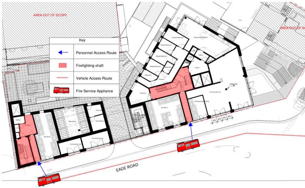
Figure 3.3 Fire Service access to ground level
