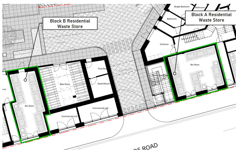
Figure 3-6 Residential Waste Store Configurations
