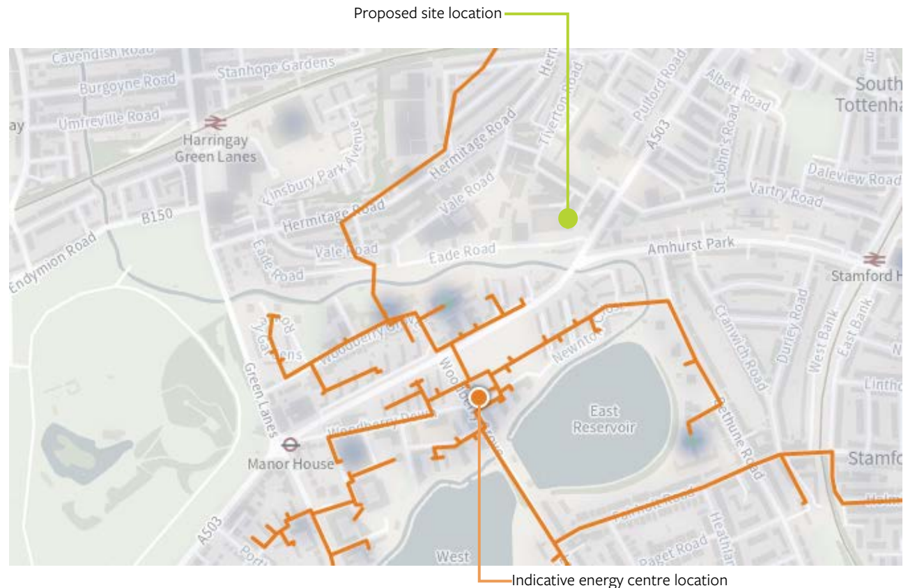
Figure 5: London Heat Map, showing proposed site location, planned Woodberry Down, Stamford Hill and Stoke Newington network and indicative energy centre location
