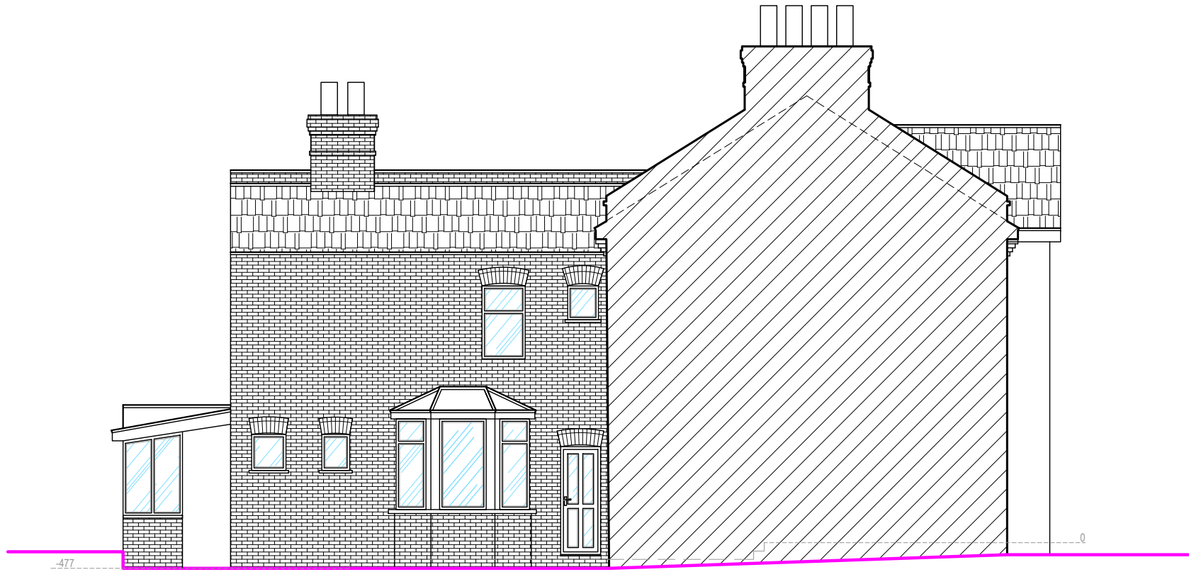
EXISTING SIDE ELEVATION 01
