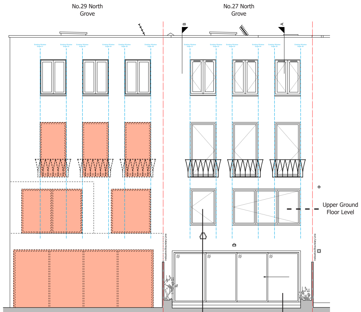
(Fig. 04) No.29 & No.27 Rear Elevation Comparison.
