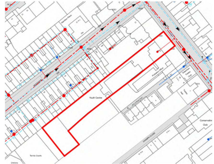
Figure 3: Extract from Thames Water Sewer Records
