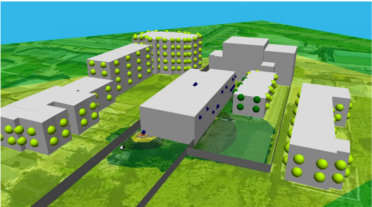
Figure 5.1: 3D Acoustic model with noise sources
