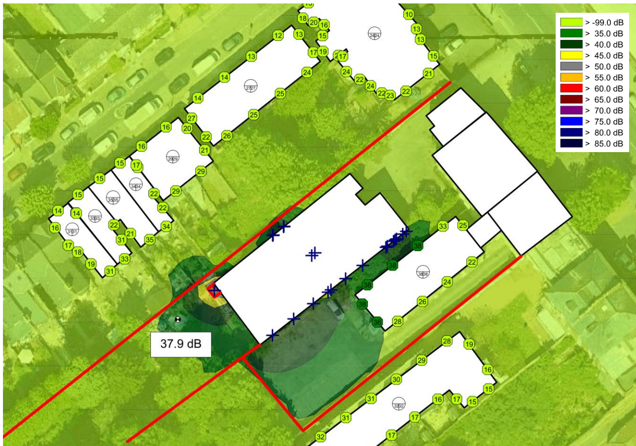
Figure 5.4: Plant noise prediction at nearest noise sensitive receivers
