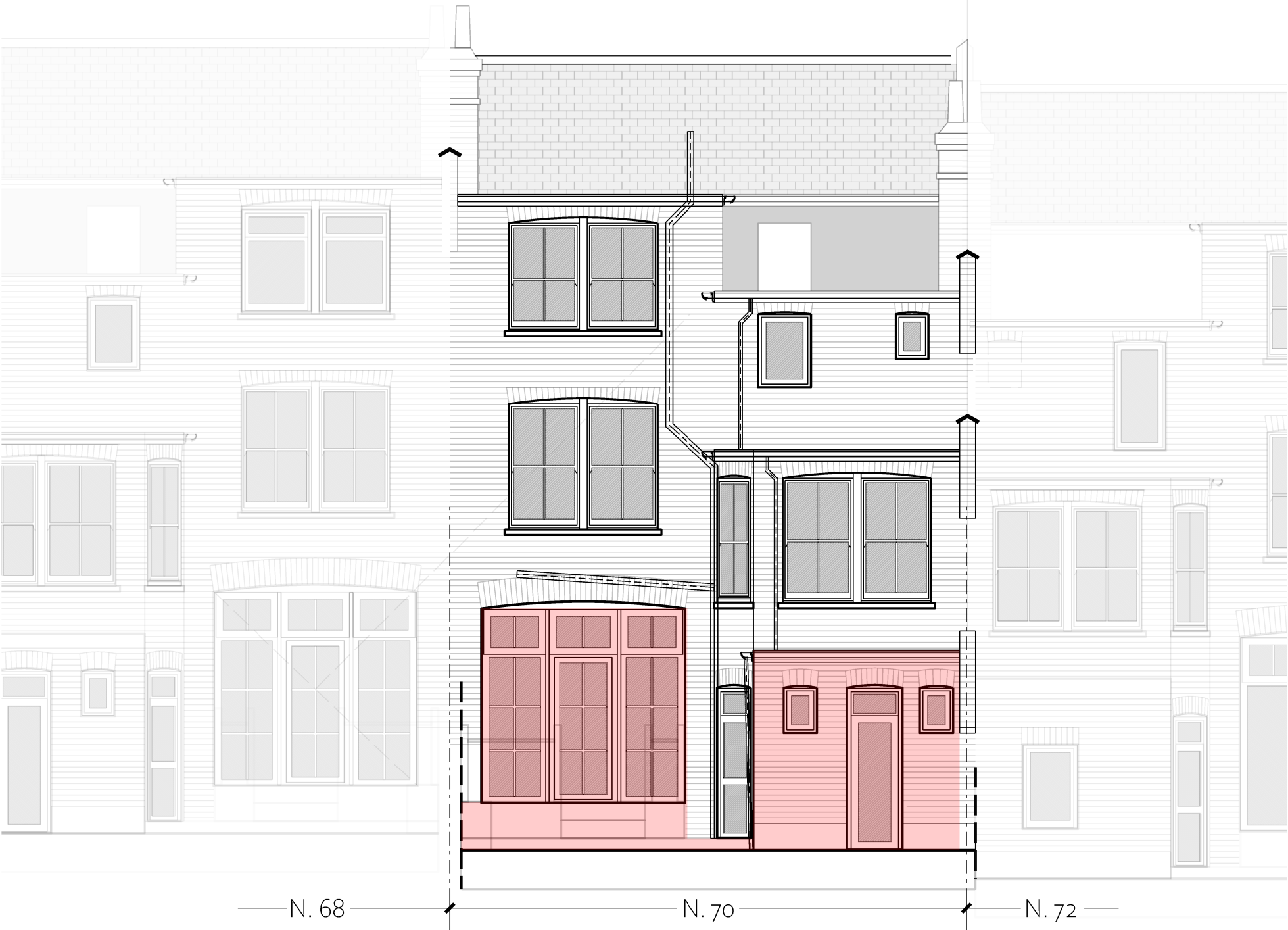
1. GARDEN ELEVATION AS EXISTING 1:200
