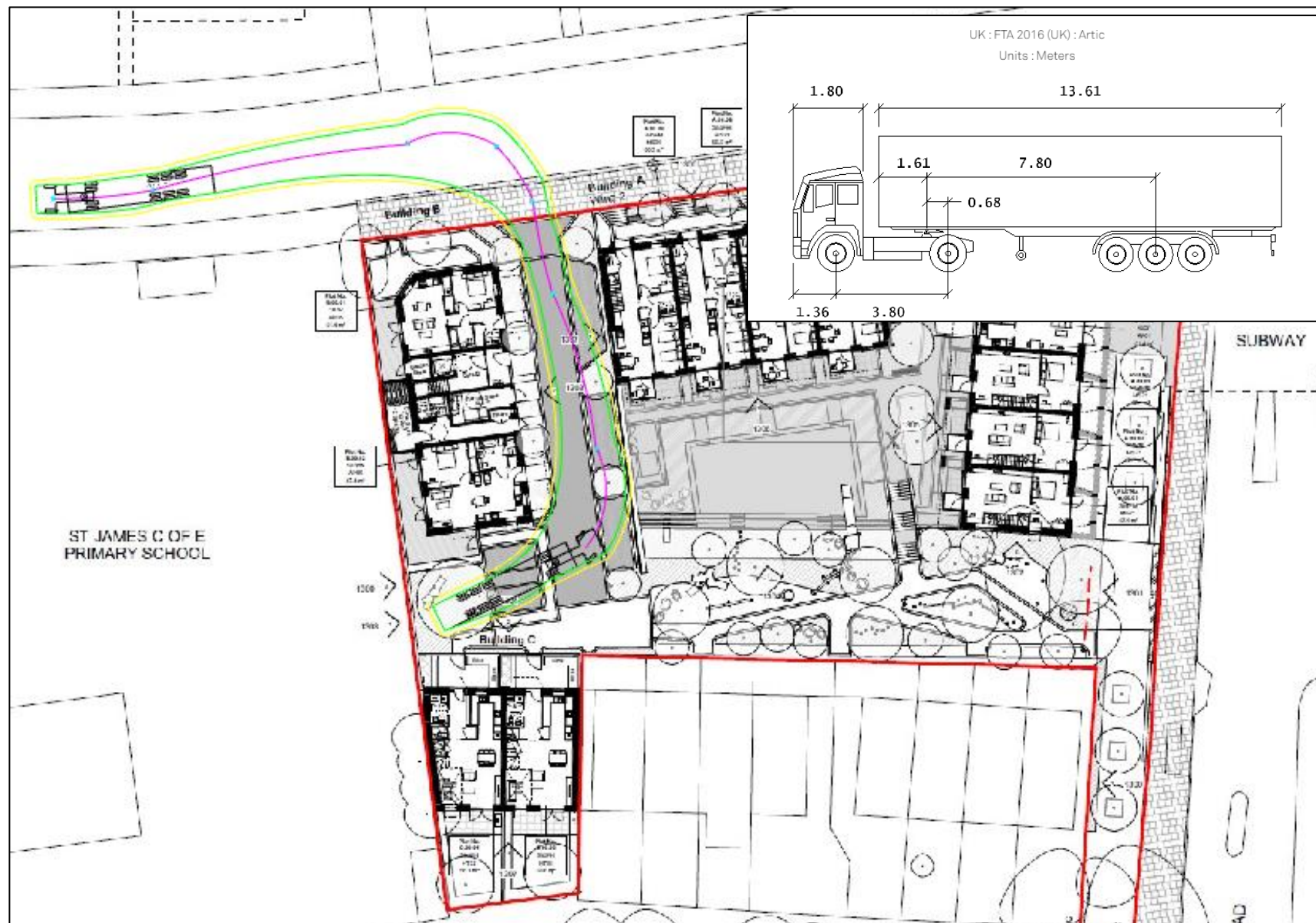
Figure 7.2(b): Construction Vehicle Egress
