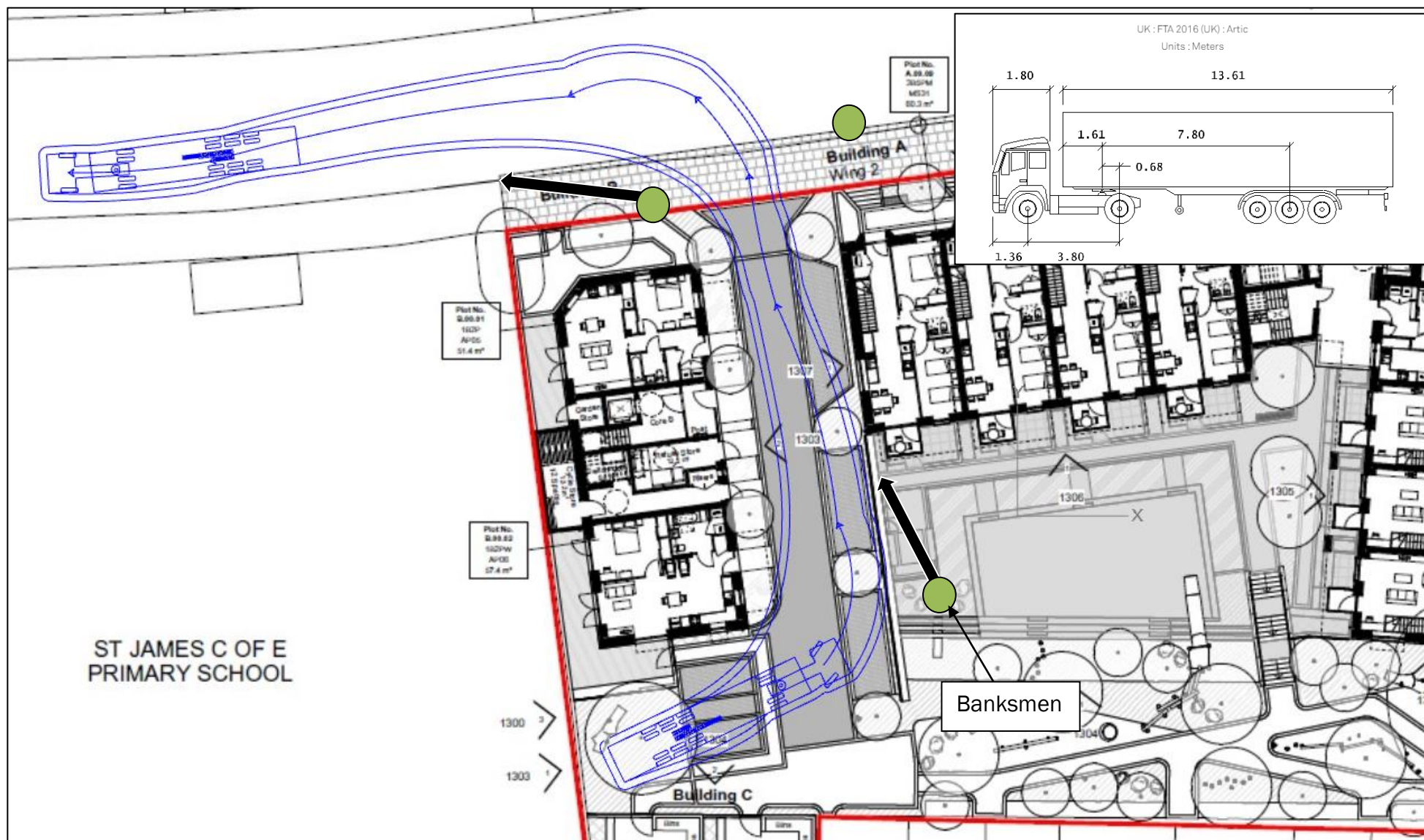
Figure 7.2(a): Construction Vehicle Egress
