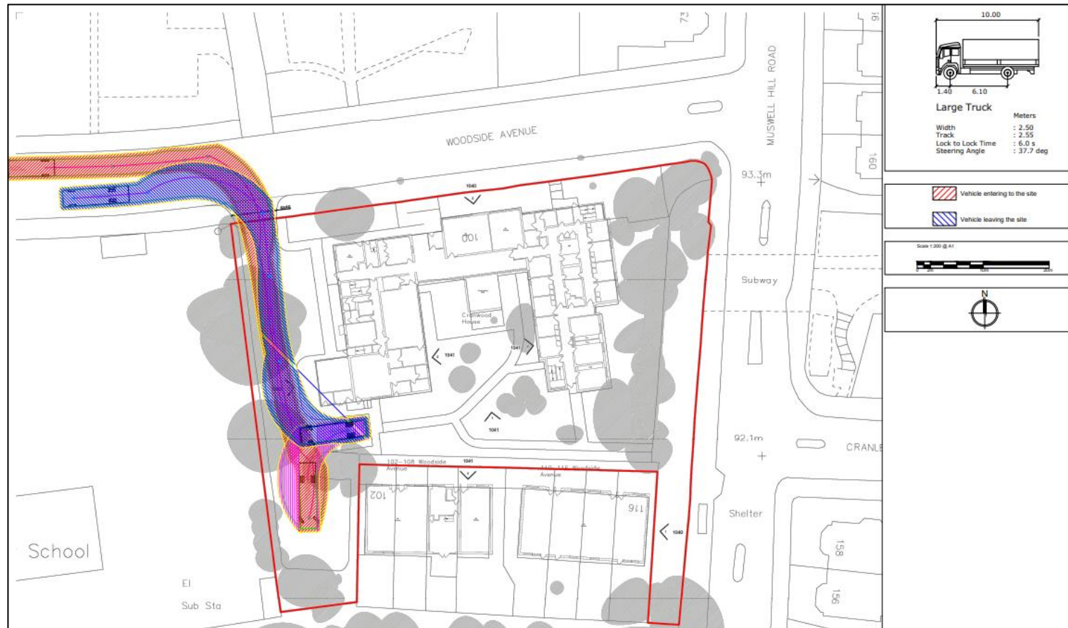
Figure 7.1: Demolition Vehicle Access and Egress (LRIGID)
