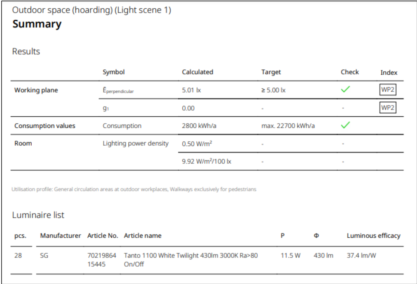
Figure 3.1: External Lighting Specification
