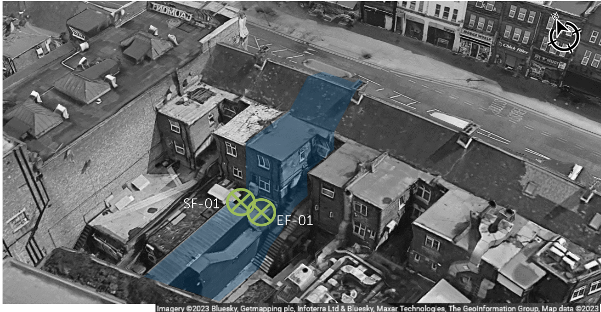
F3 Figure indicating approximate proposed plant locations
