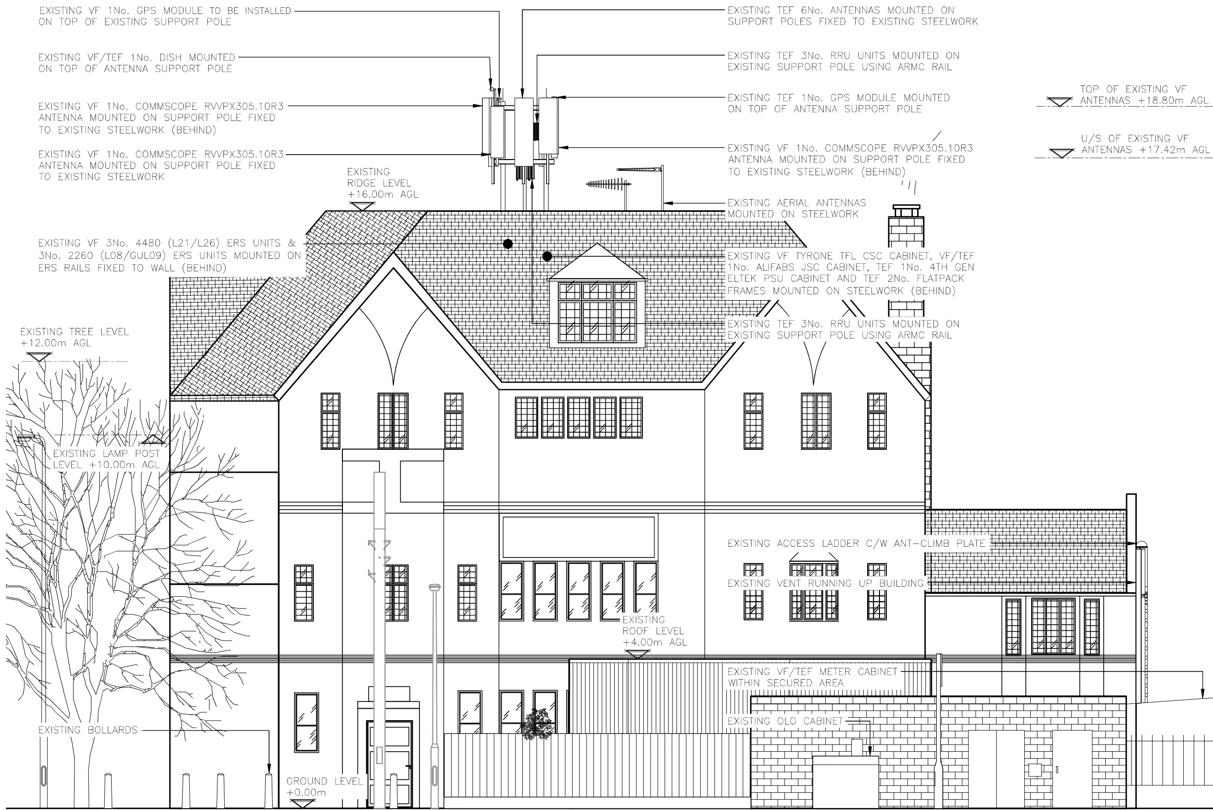
EXISTING NORTH EAST ELEVATION (1:100)
