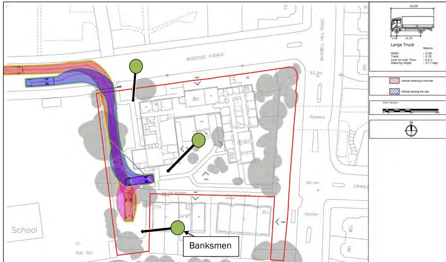
Figure 7.1: Demolition Vehicle Access and Egress (LRIGID)
