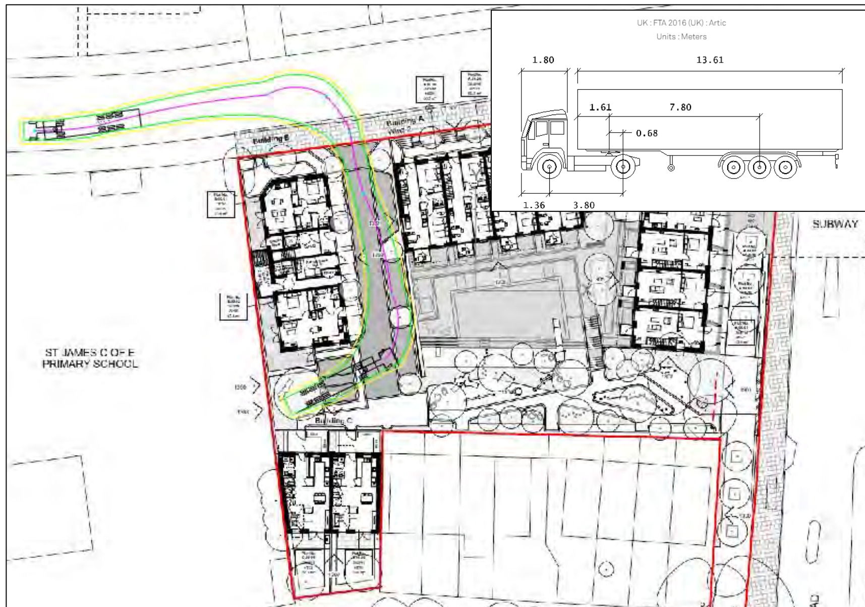
Figure 7.2(b): Construction Vehicle Egress
