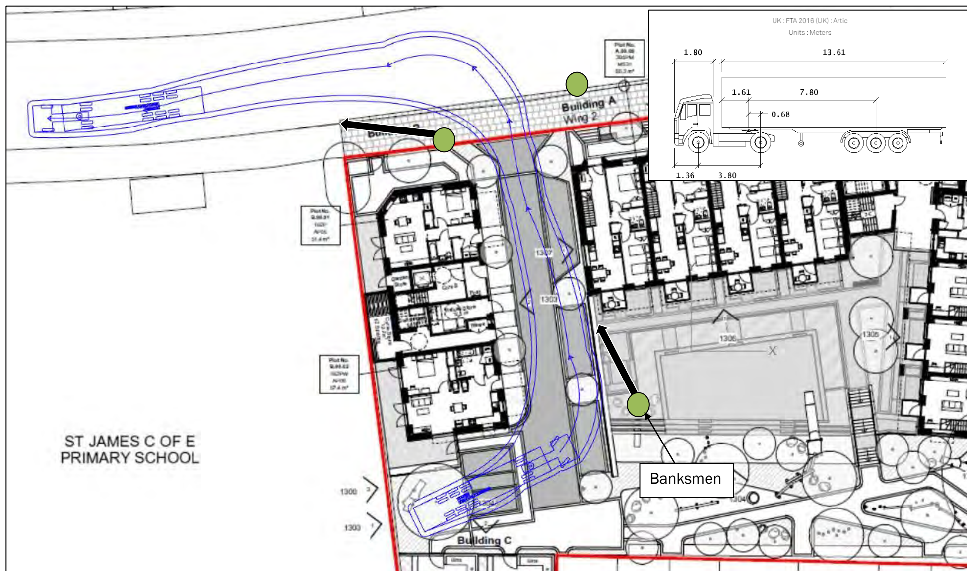
Figure 7.2(a): Construction Vehicle Egress
