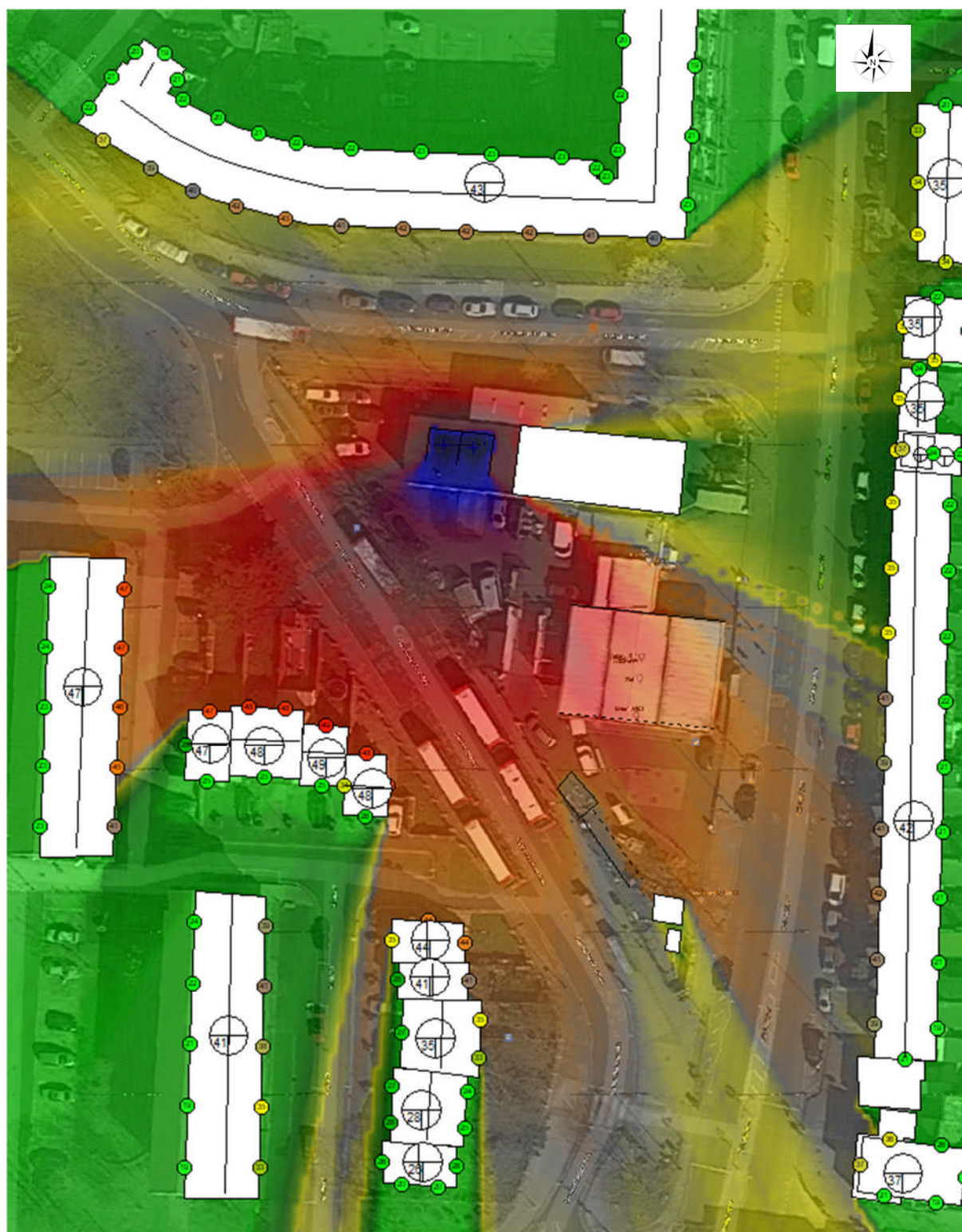
Figure 6: Specific Noise Level Calculated for the Proposed Jet Wash Bay - L_{Aeq,T}
