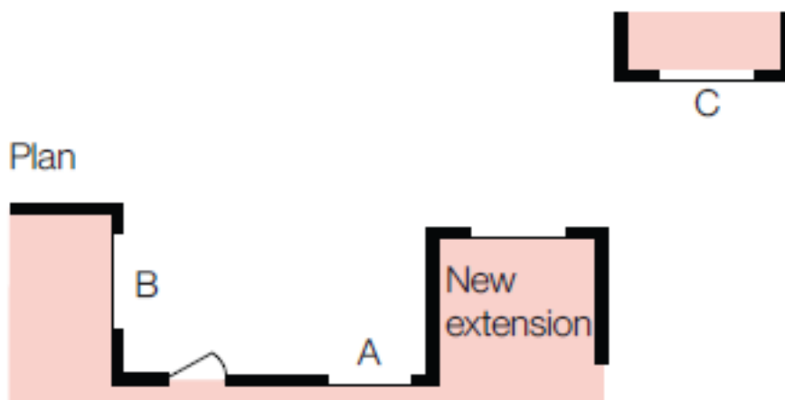
Figure 16: To assess the impact of the new extension, the 45° approach may be used for window A but not for windows B and C which directly face it
