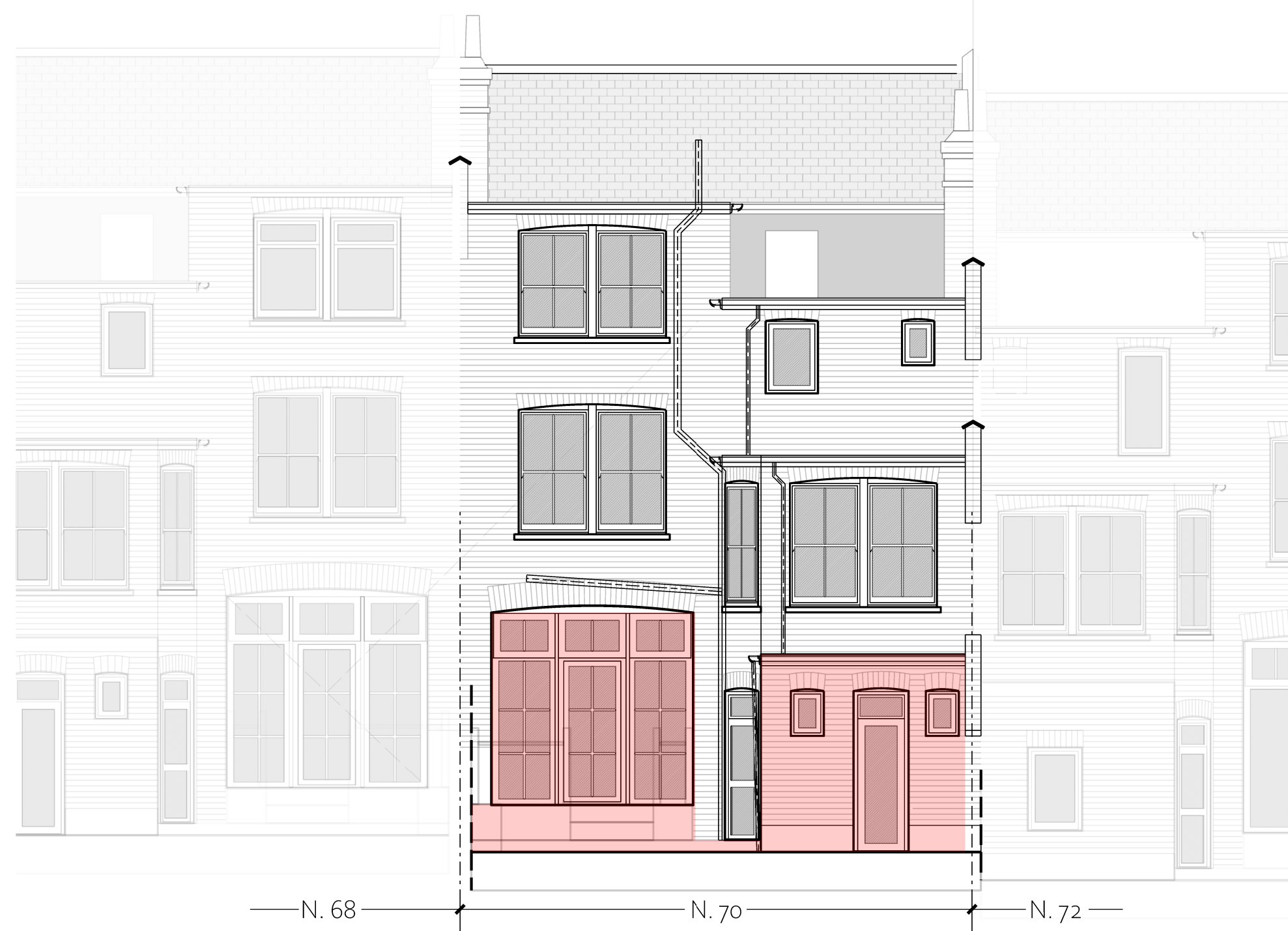
1. GARDEN ELEVATION AS EXISTING 1:200
