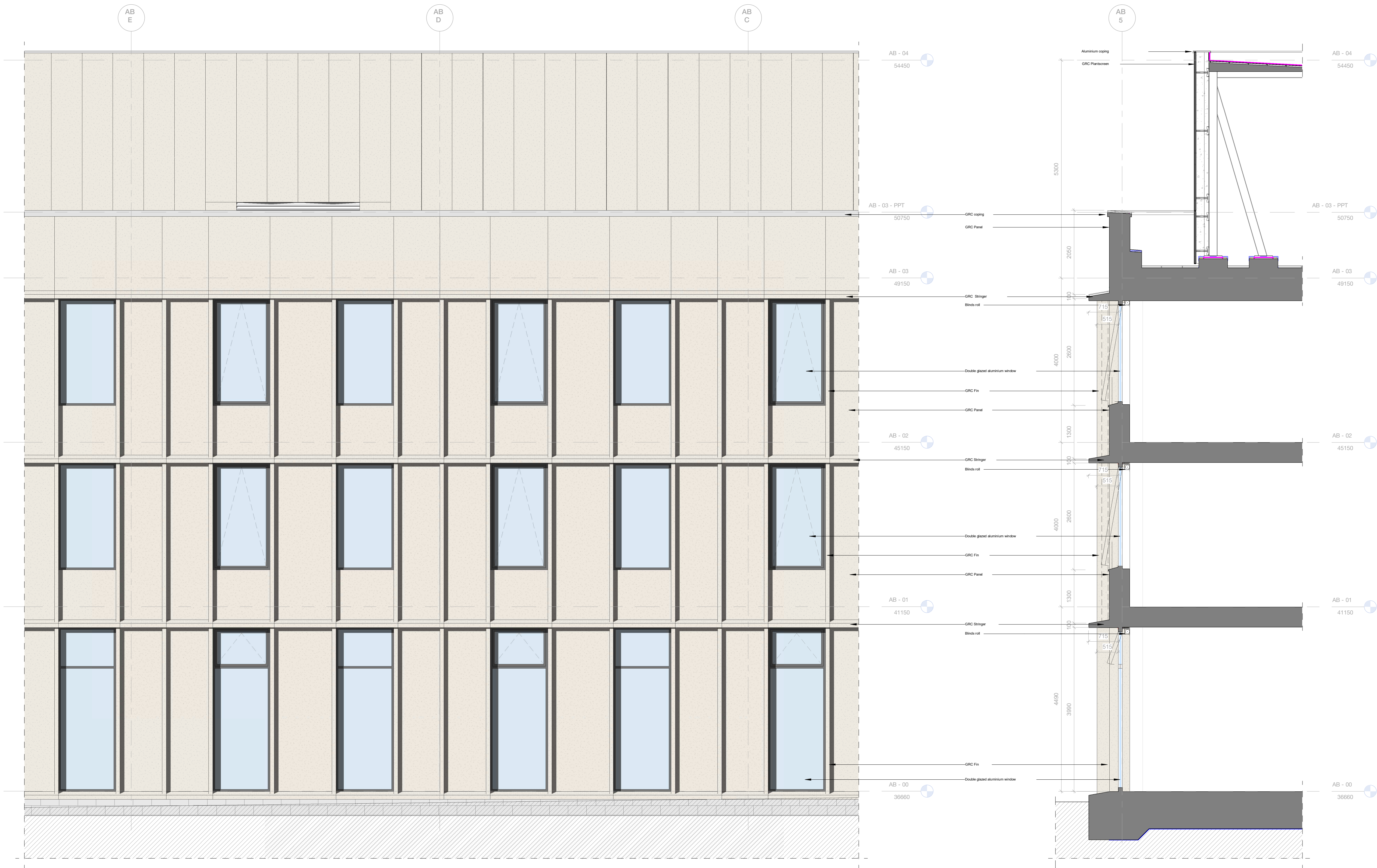
AB-ZZ-SCN N Facade Assembly Section-P 1:50
