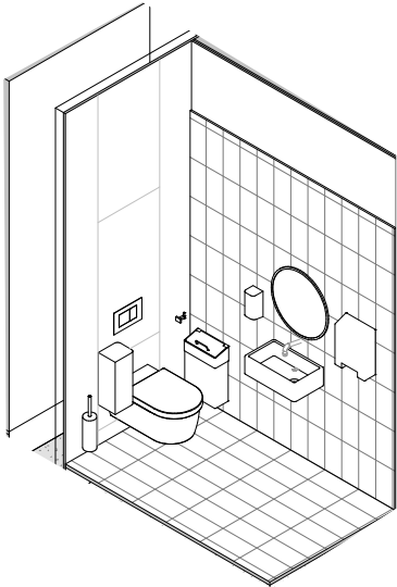
Axo of typical Toilet cubicle
