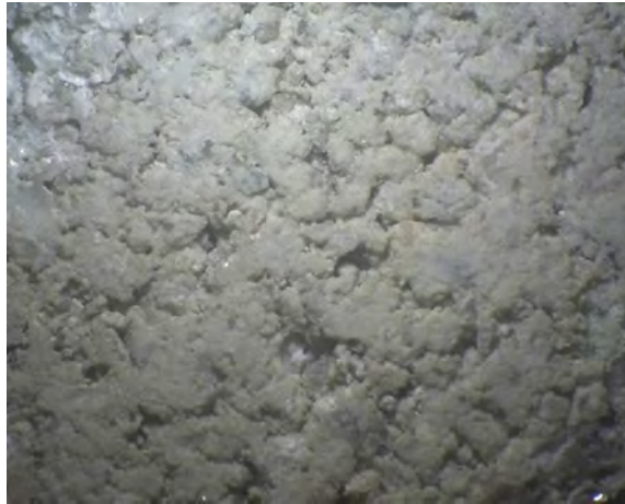
Top surface of Pre-cast stone, mag. x 60.
