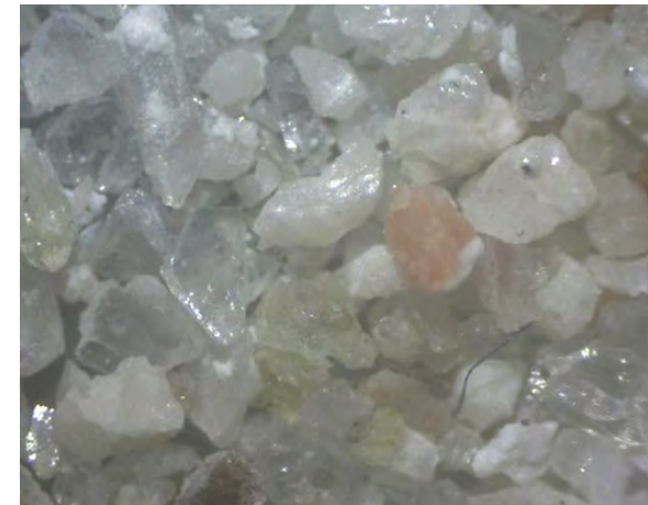
Aggregate mag. x 60. Note pinkish-white orthoclase feldspar and platelets of clear muscovite mica.
