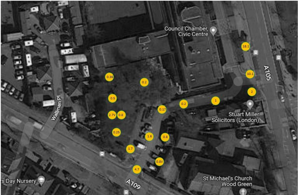
Figure 2.17 – Existing Illumiantion levels noted in values of Lux.
