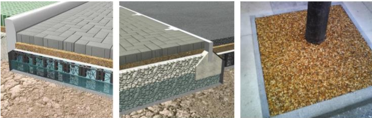
Figure 5-4 Examples of permeable surfacing.
