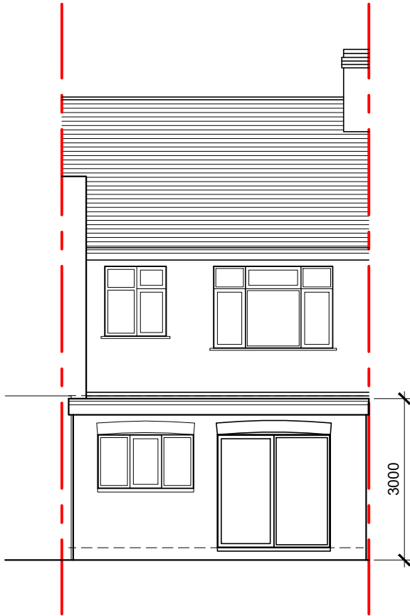
PROPOSED REAR ELEVATION SCALE 1:100
