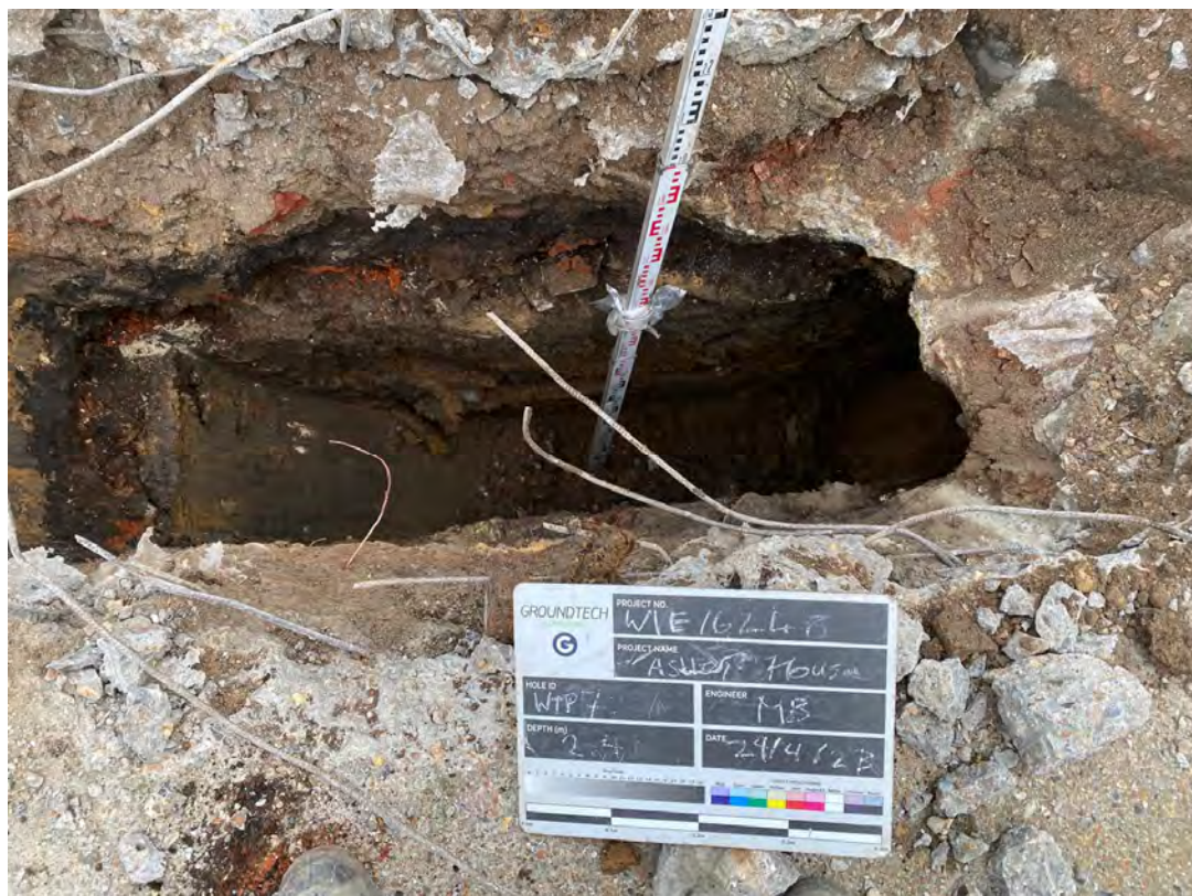
Photograph 13 – Concrete obstruction in WTP10 near underground tank.
