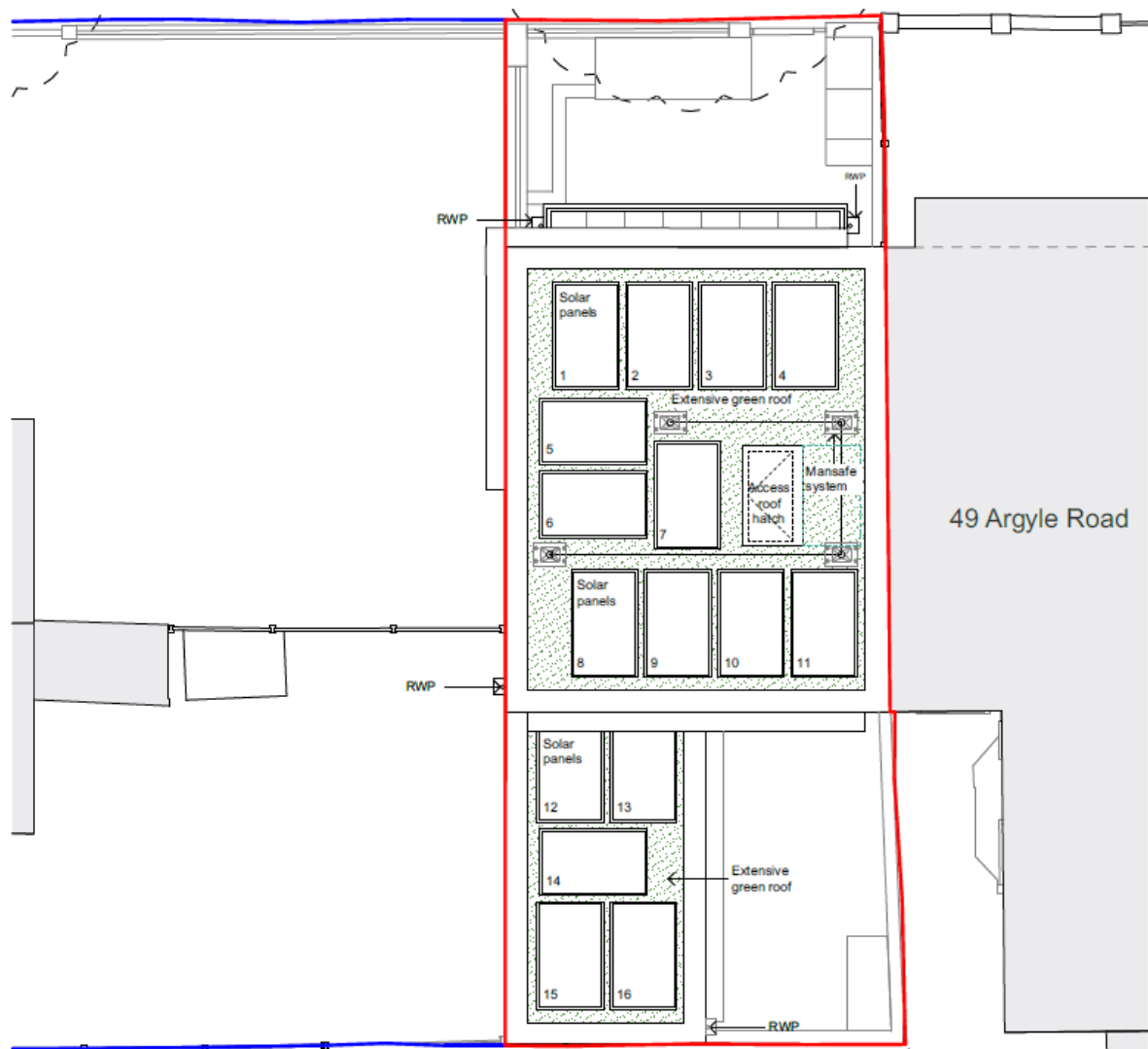
Figure 4.3 Proposed rooftop PV panel locations
