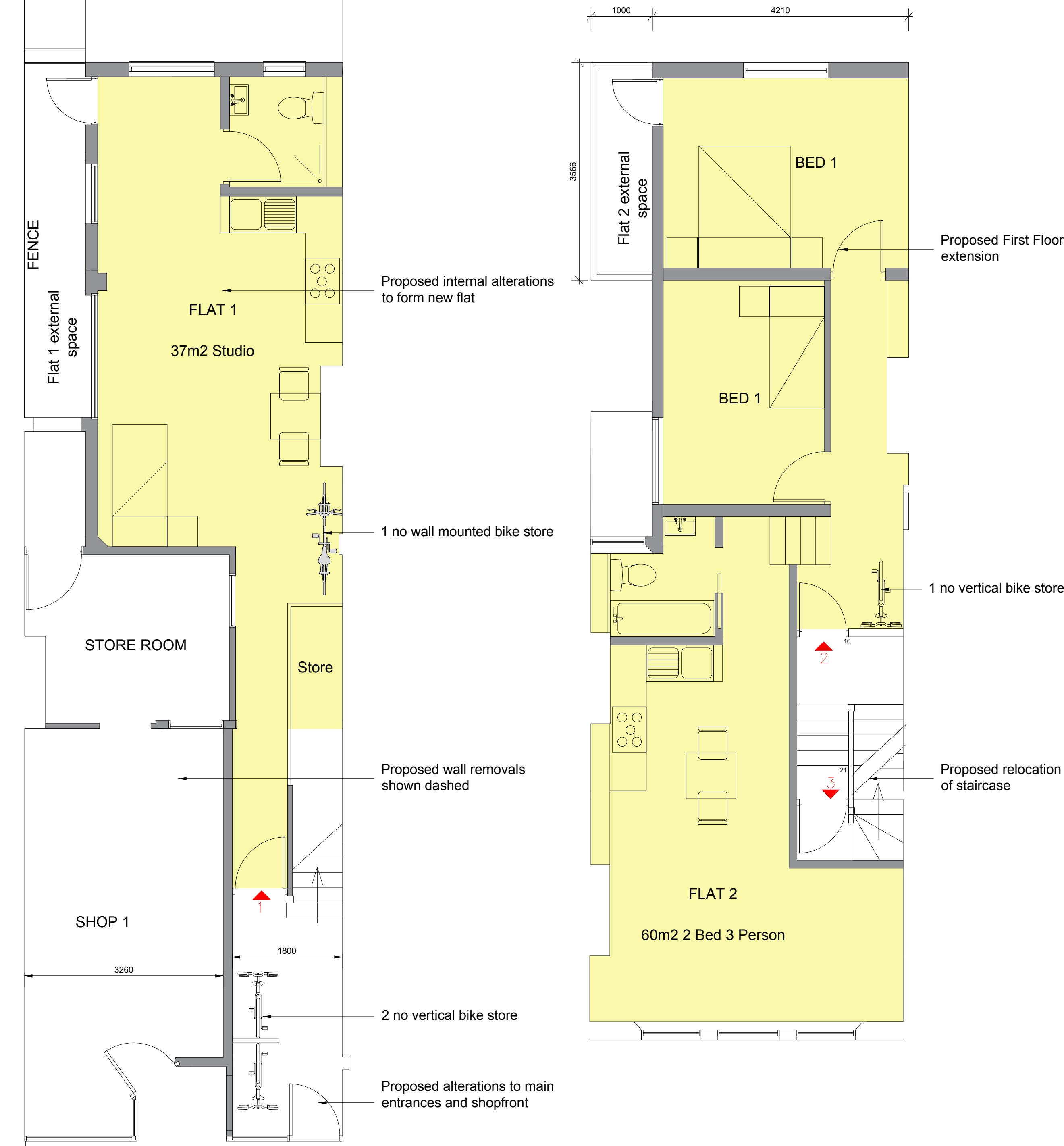
PROPOSED GROUND FLOOR PLAN
