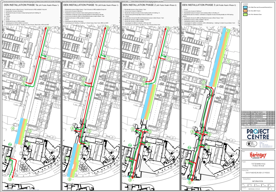
Figure 7-4 DEN phasing into site
