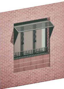
Figure 6-2 Shading design - Horizontal and vertical shading to both vertical reveals
