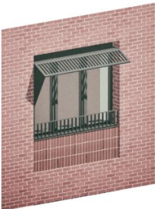
Figure 6-1 Shading design - Horizontal and southern vertical reveal
